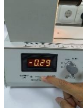
Figure 4. Changing the Display Mode to Voltage Mode.
