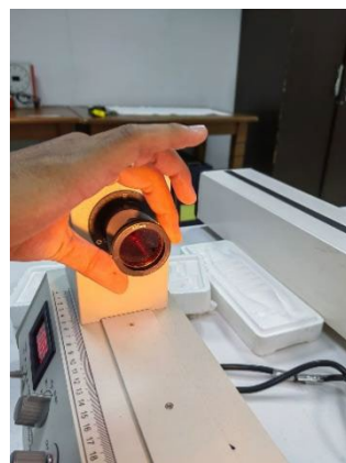
Figure 3. Experiment taking stopping potential data with a wavelength of 635 nm.
