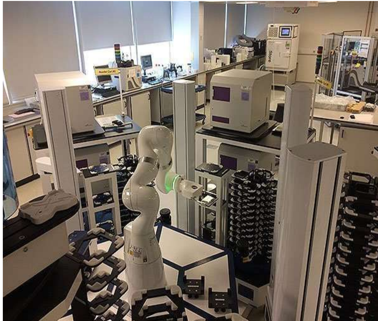
PHER Astar FSX plate readers integrated in a HighRes Biosolutions modular robotic workstation at AstraZeneca UK
