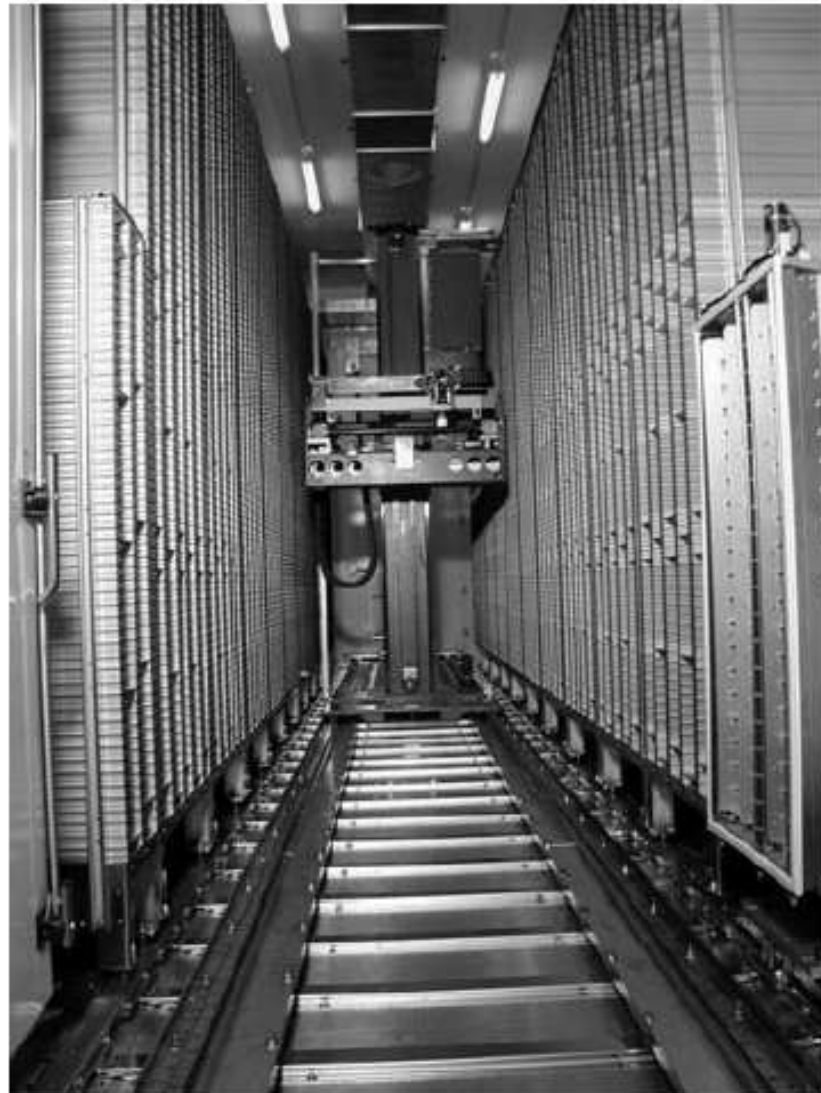
Figure 9.4.3 Liquid compound storage system with a capacity of more than 10 million deep-well sample tubes or 1.6 million microtiter plates. Robotic access enables automatic sample retrieval. (Photo reprinted with permission from REMP AG).
