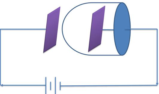
Instead of a loop, if balloon shaped surface is placed. No current passes through surface and  $I_{enc}=0$ .
