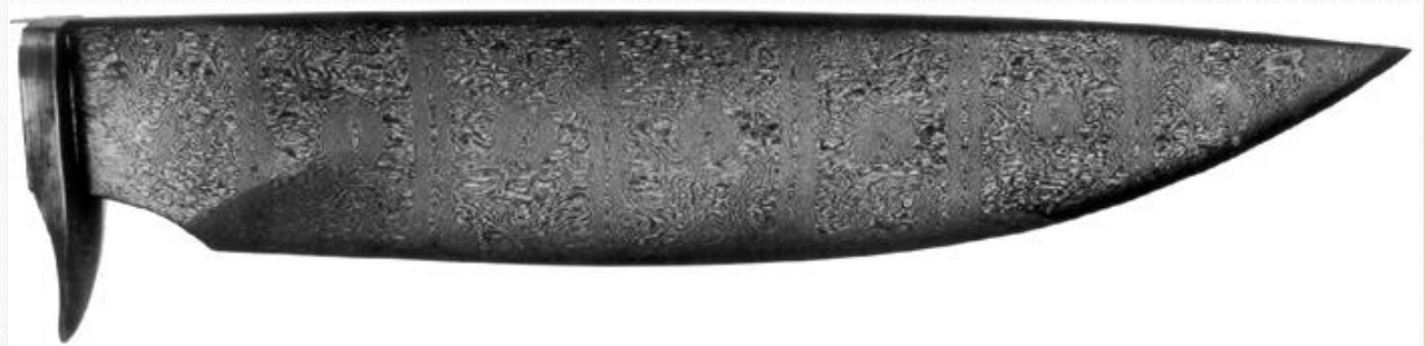
Damascus blade showing the Damascene surface pattern containing a combined Mohammed ladder and rose pattern
