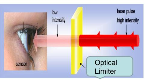
Optical limiters are SMART MATERIALS designed to have high transmittance for low level inputs while blocking the transmittance for high intensity laser beams.
